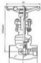
CL800 Welded bonnet, full port reducing port outside screw and yoke(OS & Y) Threaded, butt-welded or socket welded ends; design to API 602
