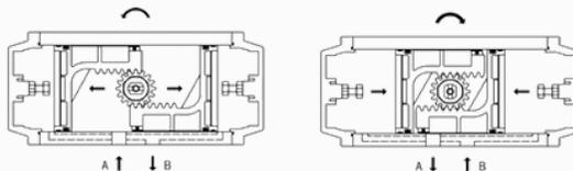
1. Air from Port A forces the pistons outwards, causing the springs to compress, the pinion turns counter-clockwise to open the valve while air is being exhausted from Port B
